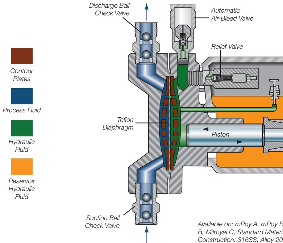
What is a diaphragm? A diaphragm acts as a seal or barrier within a pump. In a hydraulically balanced diaphragm, it is between the process fluid and hydraulic fluid that the pump is operating on. This allows for pressure to be automatically transmitted without any loss. There are also mechanically actuated diaphragms, where the piston is connected to the diaphragm. These are typically only appropriate for low pressure or limited lifetime applications.
